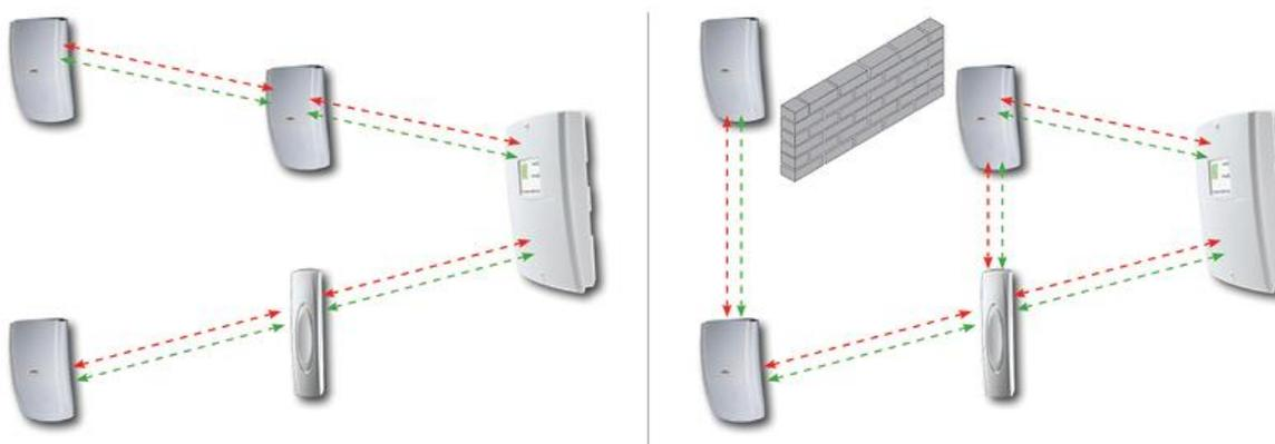
There are obvious advantages in having a wireless system, mostly associated with the fact that there are no wires to have to try and conceal in your premises, but the disadvantages are that they are typically more expensive than a Hard-Wired system, as detectors etc also have to incorporate a transmitter to communicate to the alarm control panel and their internal batteries will need to be replaced periodically, typically each year.
